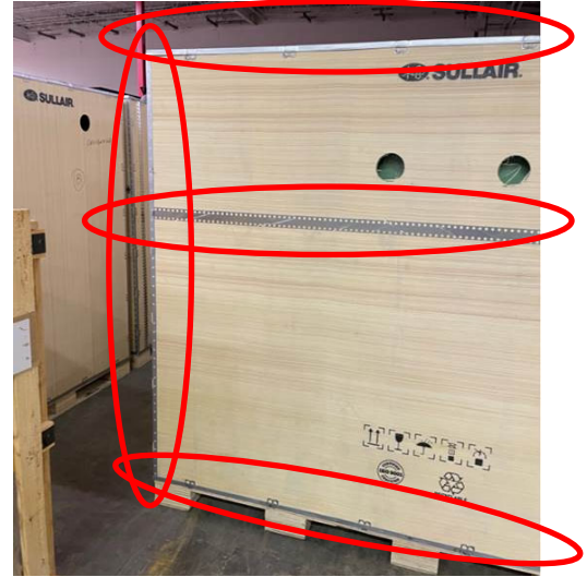
Example of strips of steel used to support the container/corners that need to be eliminated.
